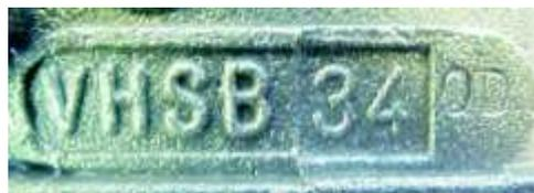
DELLORTO Type VHSB 34 (cast in carburettor body) with the letters QD or QS stamped in the body. The entire air intake shows a cast surface.
